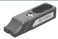
These adjustable side clamps have a low profile to keep clamp out of the way from machining operation. The clamp moves downward and forward as it is engaged, forcing the work piece against the supports and stops. Clamping surface is serrated for greater gripping strength. The body and jaw are made from SAE-4140 alloy steel, heat treated with black oxide finish.
