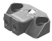
These side clamps have a low profile to keep the clamp out of the way from machining operations. Clamp moves downward and forward as it is engaged, forcing the work piece against the supports and stops. Clamping surface is serrated for greater gripping strength. Install by drilling and tapping a cap screw hole and locking pin hole. Flat washer included. The body and jaws are made from SAE-4140 alloy steel, heat treated with black oxide finish.
