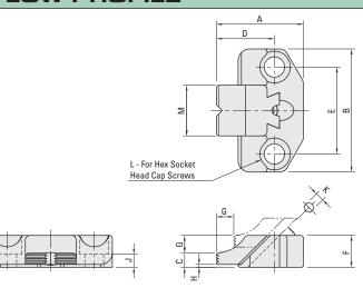
These adjustable side clamps have a low profile to keep clamp out of the way from machining operation. The serrated clamp jaws move downward and forward as it is engaged, forcing the work piece against the supports and stops. Allows for quick removal and insertion of parts. The body and jaw are made from SAE-4140 alloy steel, heat treated with black oxide finish.
