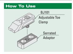
These serrated adaptors are used with the adjustable toe clamps (Series BJ101) and adjustable side clamps. (Series BJ102) They are serrated on the top to match the serrations on the bottom of the clamps. These serrated adaptors are ideal for raising the height and firmly positioning these clamps. They have a tapped hole to mount the clamps. The adaptors mount with socket head caps screws. Made from SAE-1045 alloy steel with black oxide finish.
