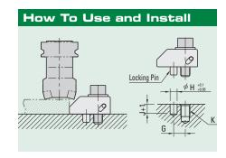
These toe clamps offer high holding power and low profile. Clamp moves downward and forward as it is engaged, forcing the work piece against the supports and stops. The low profile clamping surface is serrated for greater gripping strength. Install by drilling and tapping a cap screw hole and locking pin hole. Flat washer included. Made from SAE-1045 alloy steel, heat treated with black oxide finish.
