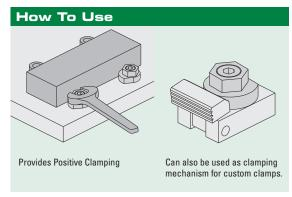
Compact design for low profile positive clamping. These clamps permit faster loading and unloading of work piece. To install, lock the flange collar into the cam using the locking screw and then tighten up the cam with a wrench. The cam and locking screw are made from SAE-4135 alloy steel. The flanged collar is made from SAE-1095 alloy steel. Parts are heat treated with black oxide finish.
