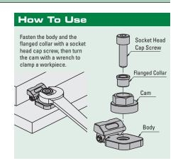
These cam edge clamps offer a low profile design, high holding forces and easy to use operations. The low profile and small size allow for faster set up and more parts per load. Turning the cam nut on the top of the clamp forces the serrated jaw forward and downward against the work piece. Easily installs with a socket head cap screw. The body and jaw are made from SAE-4140 alloy steel, heat treated with black oxide finish. The cam is made from SAE-4135 alloy steel with black oxide finish.
