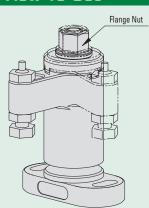
Turning the flange nut allows the arm to swing into position for clamping.
