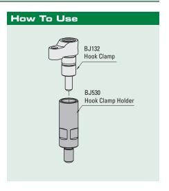
These cylindrical holders are designed for use with the compact hook clamps shown above. They provide additional clamping height as well as easy installation and operation of the hook clamps. Made from SAE-1045 alloy steel, heat treated with black oxide finish.
