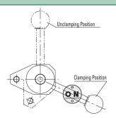
These aluminum marker plates are used to mark the handle position in the clamping mode. Pressure sensitive adhesive on the backside. 2mm holes allow for riveting. Color is red.
