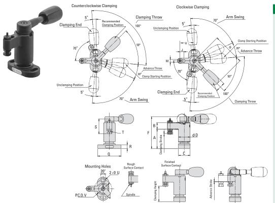
Load the work piece with the clamp arm out of the way.
