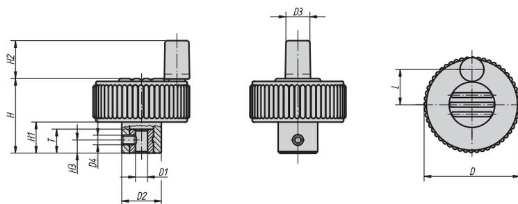
The attractive design and ergonomic features offer firm safe gripping. Made from dark grey thermoplastic. The insert is made from steel. They are available with dark grey, light grey, traffic red and bright yellow caps. See [www.fixtureworks.net](http://www.fixtureworks.net) for colors. The set screw style has a crossed tapped hole and set screw for tightening onto a shaft.
