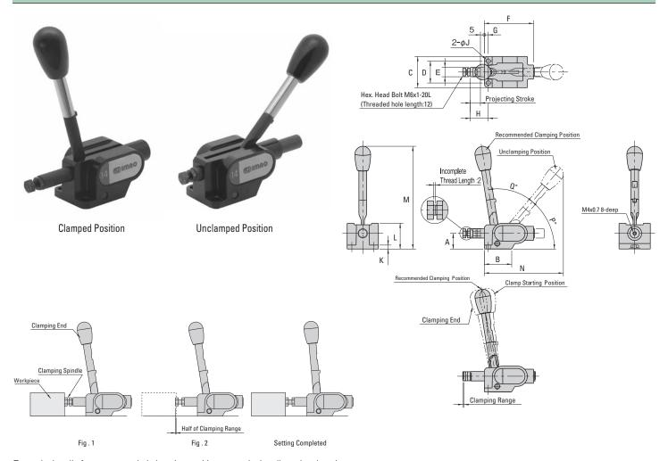
To set the handle for recommended clamping position, move the handle to the clamping position and then set the spindle to contact the work piece. (Fig. 1) Adjust the spindle by about half of the clamping range and then tighten the nuts on the spindle for locking. (Fig. 2)
