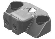
These side clamps have a low profile to keep the clamp out of the way from machining operations. Clamp moves downward and forward as it is engaged, forcing the work piece against the supports and stops. Clamping surface is serrated for greater gripping strength. Install by drilling and tapping a cap screw hole and locking pin hole. Flat washer included. The body and jaws are made from SAE-4140 alloy steel, heat treated with black oxide finish. C D Ε G
