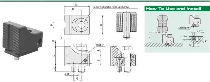
Clamp moves downward and forward as it is engaged, forcing the work piece against the supports and stops. The large clamping surface is serrated for greater gripping strength. Install by drilling and tapping a cap screw hole and locking pin hole. Flat washer included. Made from SAE-1045 alloy steel, heat treated with black oxide finish.
