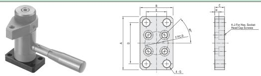
For use with the Heavy Duty Swing Clamps shown above. The plates attach to the swing clamps and allow for easy fastening and top side mounting. Can also be used to adjust the height of the swing clamp. Made from SAE-1045 alloy steel with black oxide finish.
