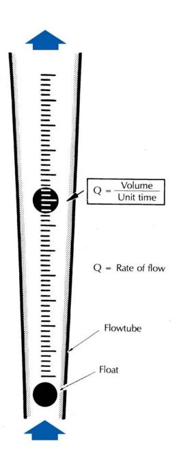
These meters have the highest useful flow ranges providing consistently reliable readings from maximum flow down to 5 to 10% of capacity. They require no electrical connections, and have low meter related pressure drops.
