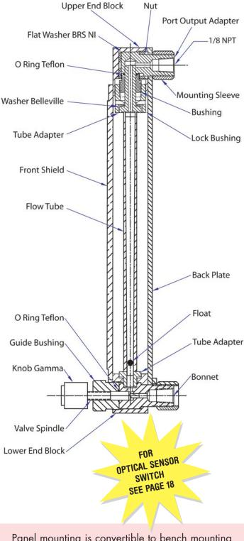
Panel mounting is convertible to bench mounting through the use of an optional acrylic tripod base with spirit leveler (catalog No. TP1).
