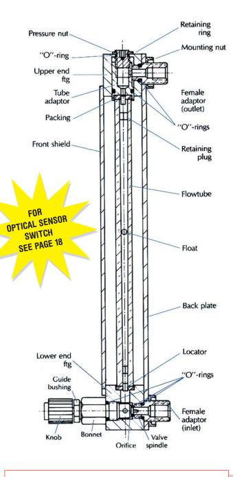
Assorted flow tubes may be used in conjunction with a single mounting frame, an apparent benefit in many laboratory applications.
