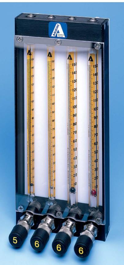
Four Tube Meter shown with MFV<sup>™</sup> Valves
