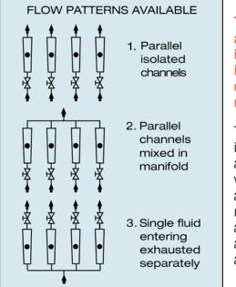
The built-in-valves are always installed in the end block opposite to the manifolded one.
