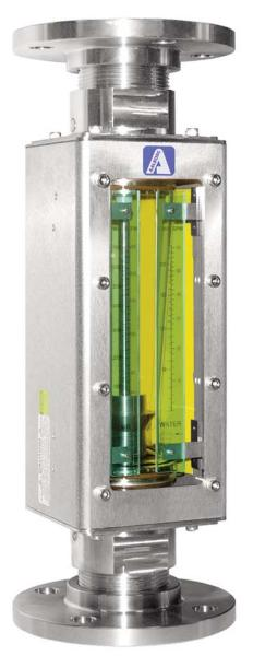
Meters are graduated for direct reading of water and air. Flow meters come with FNPT or flanged end fittings for easy in-line installation. Wetted parts include borosilicate glass flow tubes, Viton<sup>®</sup> o-rings, and 316 Stainless steel fittings, guide rods, floats and float stops. <image>
