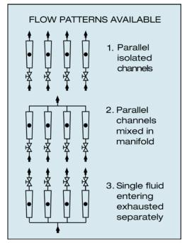
When meters with valves are ordered the valve cartridges are installed at the inlet.
