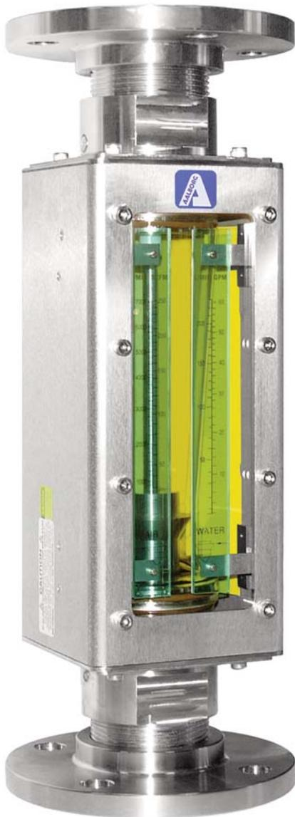
Meters are graduated for direct reading of water and air. Flow meters come with FNPT or flanged end fittings for easy in-line installation. Wetted parts include borosilicate glass flow tubes, Viton® o-rings, and 316 Stainless steel fittings, guide rods, floats and float stops.
