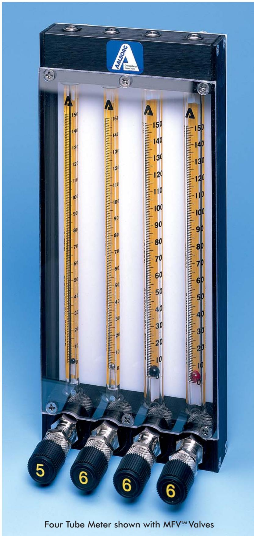
Four Tube Meter shown with MFV™ Valves
