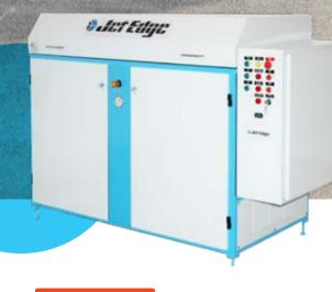
he IP60-30 is designed for shops that desire the reliability of a hydraulic intensifier pump, but have limited power. This pump is capable of producing 0.6 gpm (2.3 lpm) of UHP water at a continuous operating pressure of 55,000 psi. It includes a hydraulic accumulator to provide smoother hydraulic pressure, reduce spikes, and prolong hydraulic pump life.
