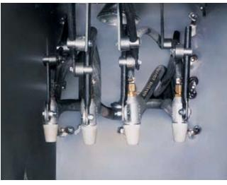
Four suction-blast guns, mounted on adjustable holders, enable operators to control blast coverage.
