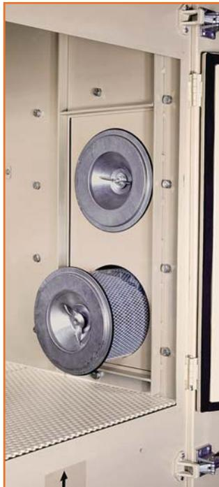
ProFormer cabinets are equipped with cartridge-type dust collectors to facilitate a quick change of filtration surfaces. These two cartridges have a filtration area of 103 square feet each, providing a total of 206 square feet, and can be replaced in minutes through the cabinet door. As a result, loose dust falls into the cabinet rather than onto the work floor.
