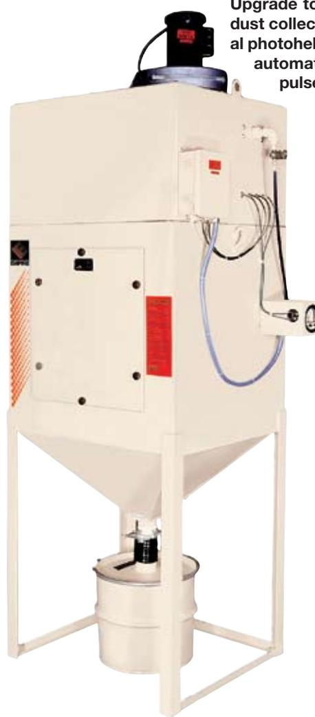
Upgrade to cartridge-type dust collector with optional photohelic package that automatically controls pulse-jet cleaning
