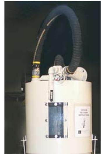
Floor hopper, including a trash-removal screen, facilitates media recovery on work sites and within custom blast enclosures. Hopper may be recessed in pit for sweep-in collection of abrasives.
