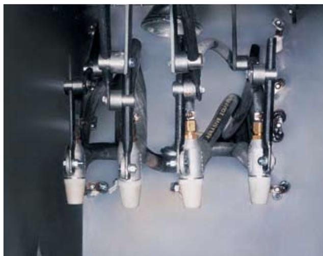
Four suction-blast guns, mounted on adjustable holders, enable operators to control blast coverage.
