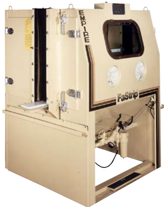
This pass-through cabinet simplifies the handling and finishing of metal or glass plates. Special features include a gasketed entrance/exit slot between the cabinet's double doors in addition to interior part guides that facilitate material handling.
