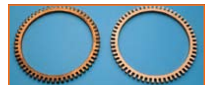
Collar deburred with glass beads
