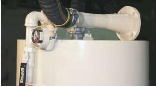
Empire's Vacutrans<sup>TM</sup>, a high-velocity venturi head, enables retrieval of media at rates exceeding 8,000 pounds per hour. Optional silencers and exhaust-hose extensions are available for sound attenuation.
