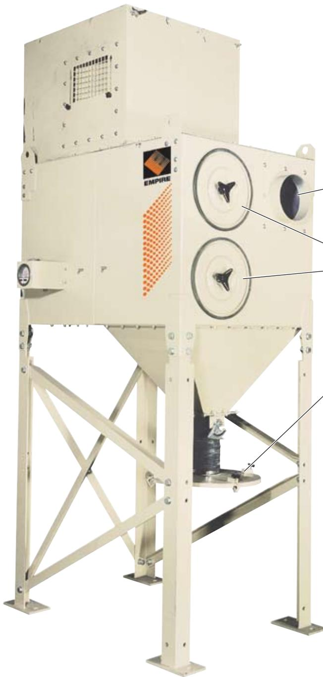
Designed for dust collection with high-production equipment, such as automated air-blast systems, these EM cartridge collectors increase air flow, provide more filtration area and clean filters automatically.
