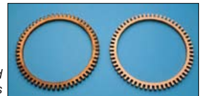
Collar deburred with glass beads
