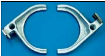
Shifter forks etched with ALOX
