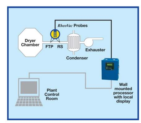
The probes are installed in the vacuum line, downstream of the process. The *RheoVac DR* provides a continuous stream of data for evaluating the performance of the dryer system. The rates of removal of water vapor and purge gases can be measured separately, if required. The operator can view the information locally by scrolling between the output parameters on the wall-mounted processor. This information can also be transmitted to the plant control room for review.
