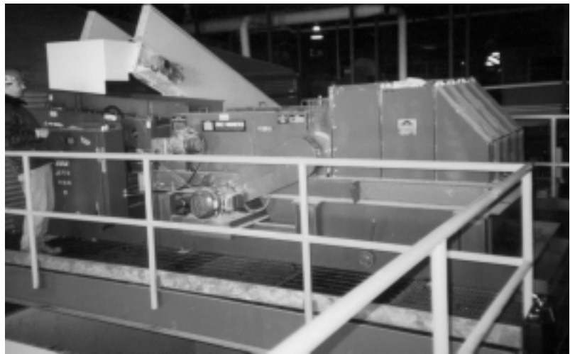
ECS-24" REA, Type M Removing used beverage cans (UBC) from household trash
