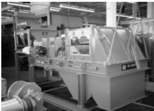
ECS-24" REA, Type PET with Hopper and Feeder Removes small aluminum contaminants and purifies PET (plastic) flakes. An RE Roll Magnet fitted to the right side removes weakly magnetic contaminants.
