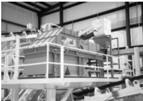
ECS-24" REO, Standard Removing aluminum from glass cullet
